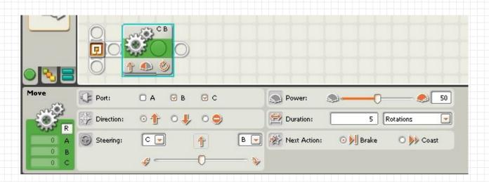
Moves two motors simultaneously
